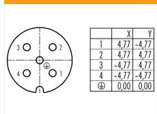
Contact arrangement (Plug-in side)
